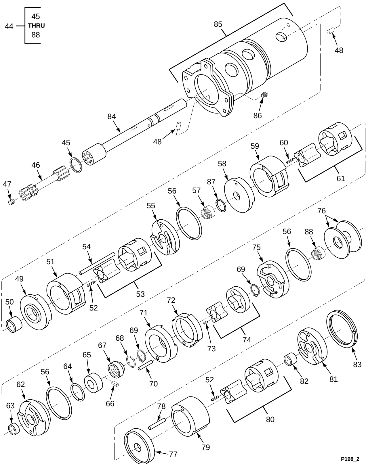
FIGURE 198. PUMPING UNIT, HYDRAULIC (SHEET 2 OF 2)
